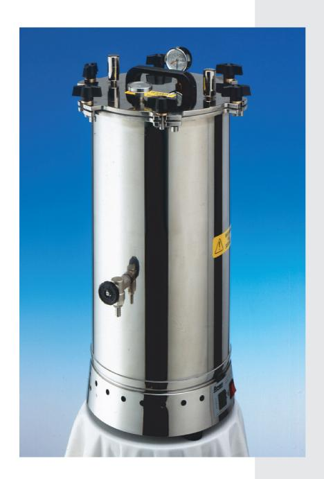
Compact and Fully Portable **Electronic Temperature Control** Simple and Safe Use **Domestic Electricity Supply** No Plumbing Needed Minimal Maintenance Required Electrically Safe To BS3456 Lid Locking Safety to H&SE PM73 Produced under ISO 9001 Suitable for Culture Media 121°C Operating Temperature 316 Stainless Steel Construction 30 Litre Capacity 280mm Internal Diameter 23.0Kg Net Weight **CE Marked**
